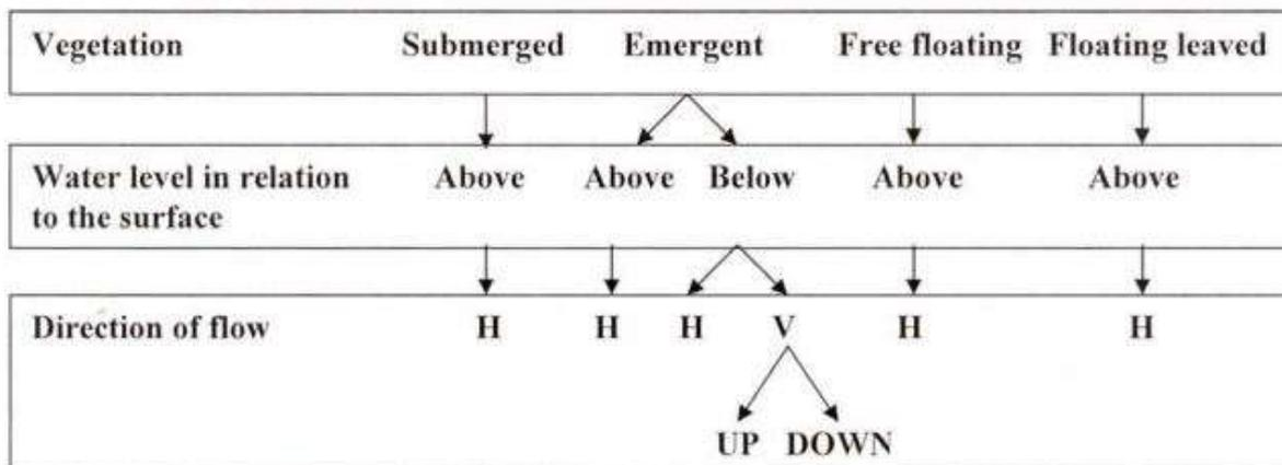
Figure 1: CW types for pretreatment of wastewater (H=Horizontal, V=Vertical)
