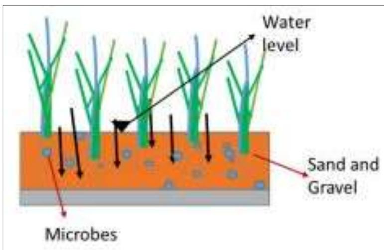
Figure 7: VSSF Schematic
