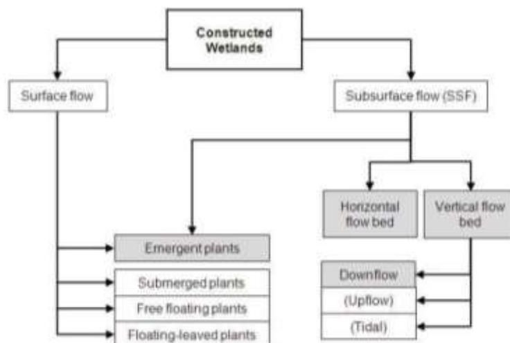
Figure 3. Classification of constructed wetlands
