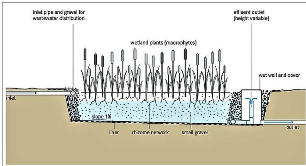
Figure 6: HSSF Schematic [20]
