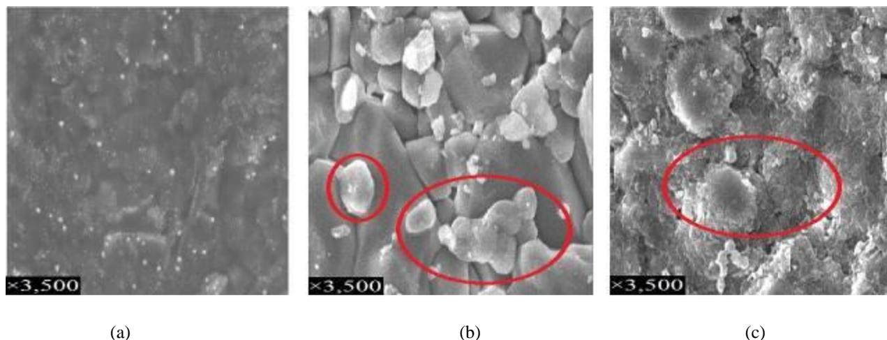
Figure 4. SEM images of SPCE surface. (a) Clean surface of working electrode (Oviedo, Spain). (b) Bacteria bound before measurement for 3 days. (c) Biofilm matrix of bacteria bound after measurement for 35 days
