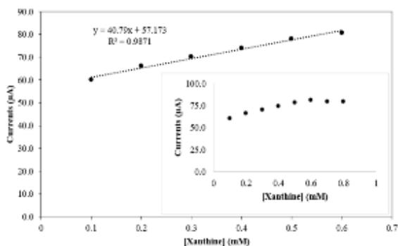
Figure 6. The linearity curve of xanthine concentration to the current response. Inset is when the substrate fulfills all parts of active site enzyme at 0.6-0.8 mM of xanthine concentration
