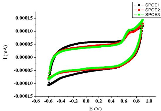
Figure 9. Voltammogram repeatability of optimum condition of the antioxidant biosensor
