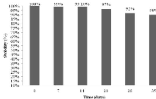
Figure 8. Stability of biosensor antioxidant since 35 of days
