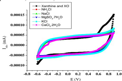
Figure 7. Voltammogram of selectivity measurements against interferen ions
